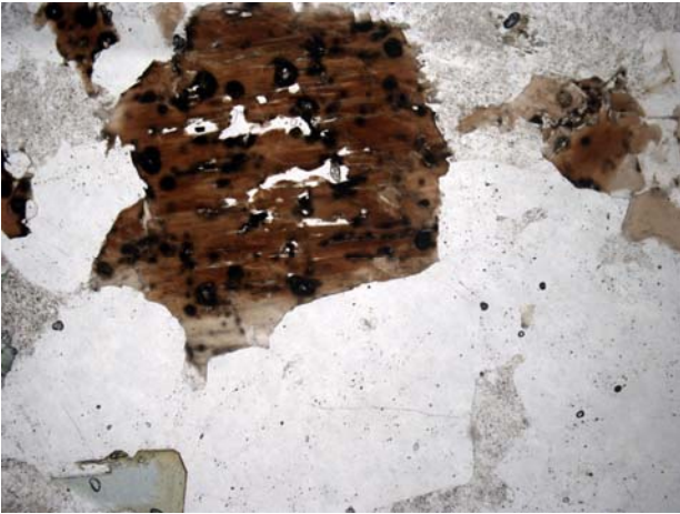
Plate 6. Dartmoor sample (M1378), with circular pleochroic halos in biotite (brown) from the radioactive decay of small zircon crystals.
