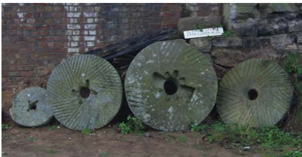
Plate 1. Old millstones at Daniel's Mill, Bridgnorth. From the left: (a) 25 in. (0.64 m) granite runner stone with straight (cruciform) rynd mortise (7); (b) 41 in. (1.04 m) dia. granite runner with curved rynd mortise (8); (c) local sandstone with mortises for wooden and iron rynds, possibly from Hexton's Quarry, near Upper Arley; (d) 42 in. (1.07 m) granite bedstone (9) for use with (8).
