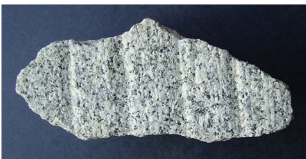
Plate 2. Fragment of granite millstone (16) found at New Hall Mill, Sutton Coldfield, showing minerals and texture. White regions are feldspars, whereas quartz is colourless, and the black areas are mica. Note asymmetric furrow cross-section.
