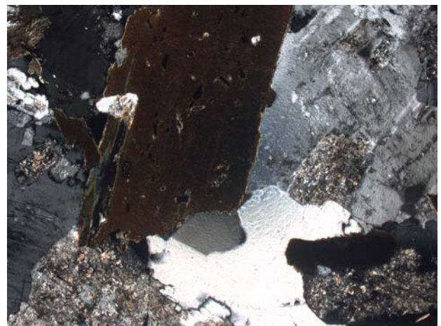
Plate 5. Cooper's Mill (6), showing partial breakdown of biotite (brown) to chlorite.
